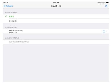
Press to select the Network Audio Interface input stream you would like to associate with the inputs you have chosen. (In this case, you are assigning Input 1-16). The selected input for this bank is now displayed in green with a checkmark to its left.
